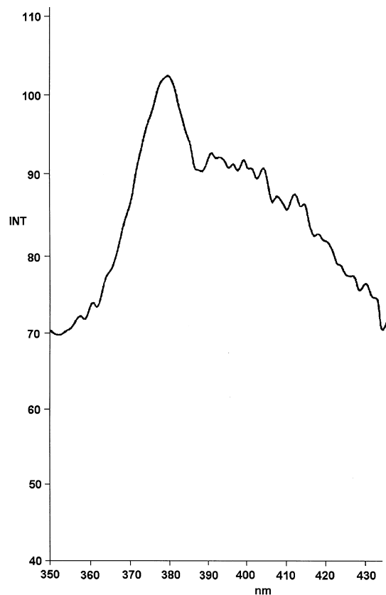
Fig. 1. Luminescence spectrum of rat skin collagen obtained at 340 nm excitation.
